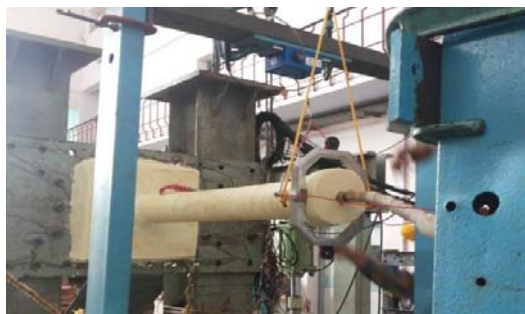
Fig.6 Test set up for cantilever loading of polyimide pipeline
